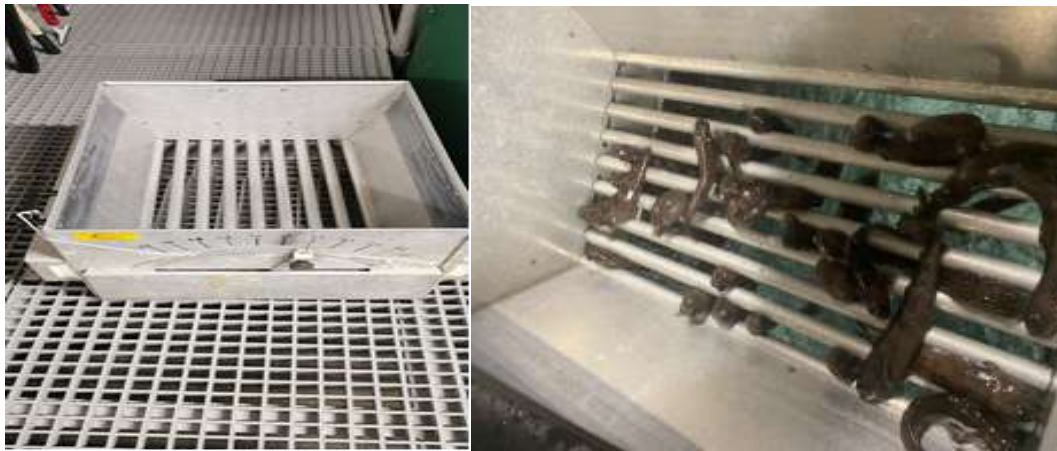
Figure 22: Box grader used to grade smaller wolffish
