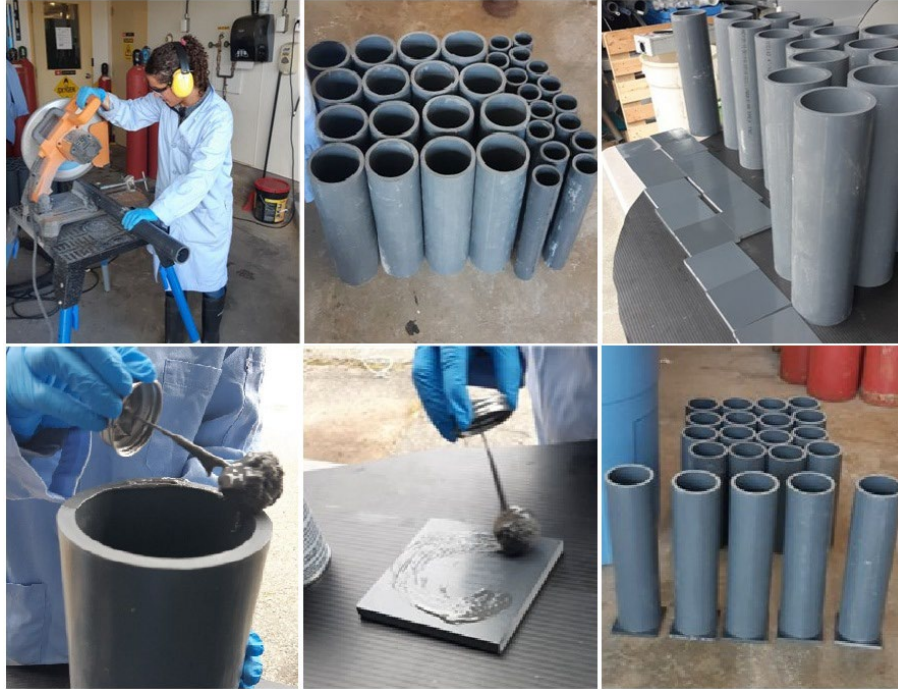
Figure 3 - Settling tube crafting. Top L to R: PVC piping being cut to size and prepped for base assembly. Bottom L to R: Cement being applied to settling tube and base, assembled settling tubes left to dry.
