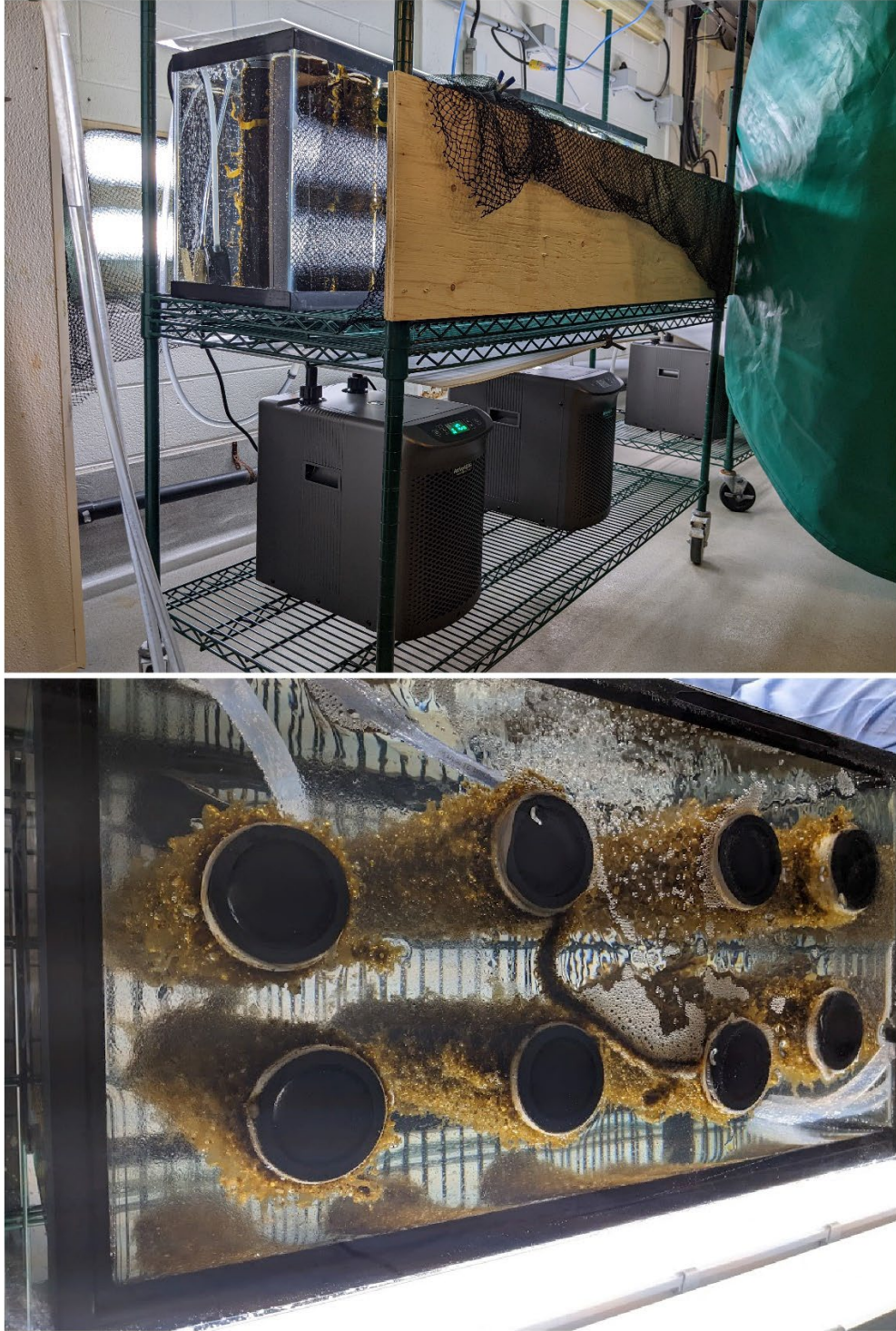
Figure 2 – Assembled seaweed nursery. Top: Front view of nursery setup with rack, chillers, tanks, and lighting panel. Bottom: Over head view of spools in tank.
