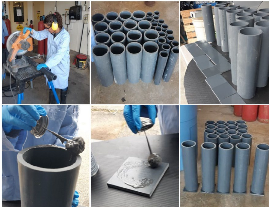
Figure 4 - Settling tube crafting. Top L to R: PVC piping being cut to size and prepped for base assembly. Bottom L to R: Cement being applied to settling tube and base, assembled settling tubes left to dry.
