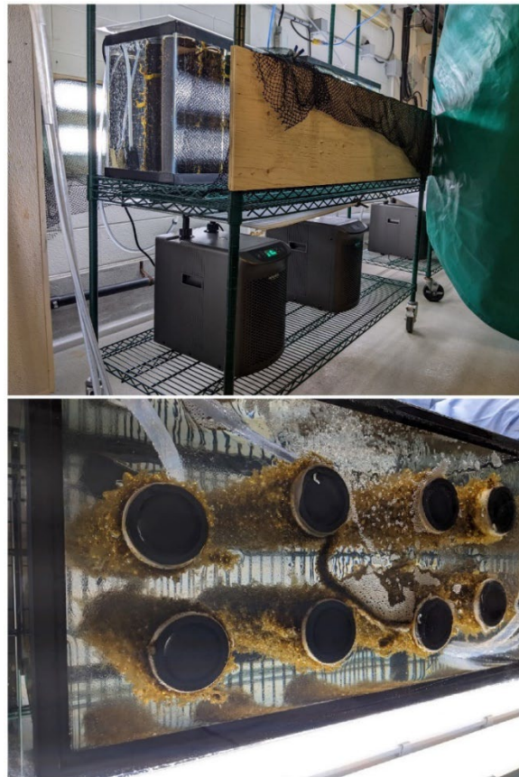
Figure 3 - Assembled seaweed nursery. Top: Front view of nursery setup with rack, chillers, tanks, and lighting panel. Bottom: Over head view of spools in tank.
