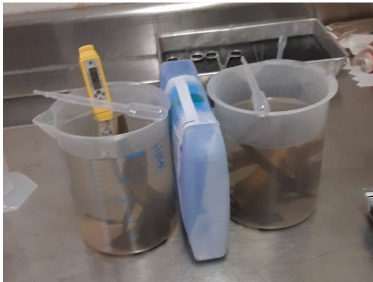
Figure 10 - Sorus placed in saltwater with nutrients for spore release.
