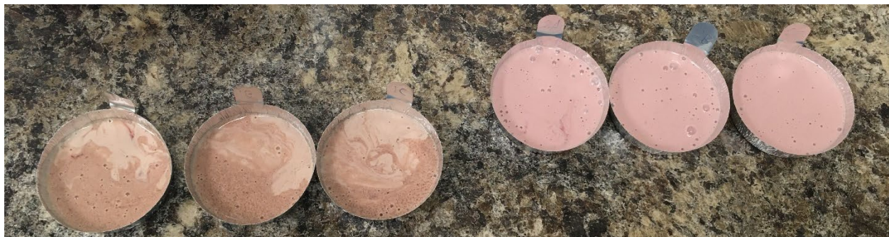
Figure 9: Moisture analysis of blended raw material. SMP 1 (left) was frozen for 7 days while SMP 2 (right) was frozen for 1 day only – oil release is happening in the older sample while no oil separates from the 1-day old sample
